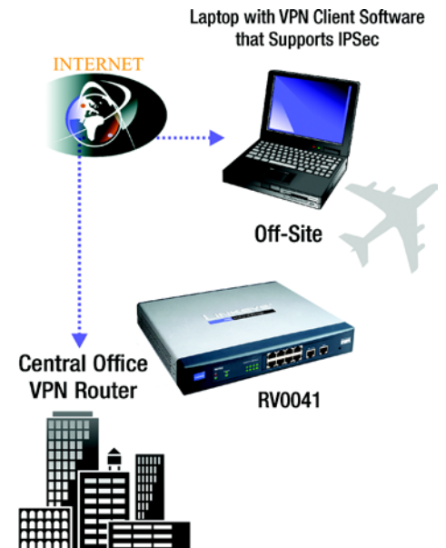
Figure 2-2: Computer-to-VPN Router VPN
